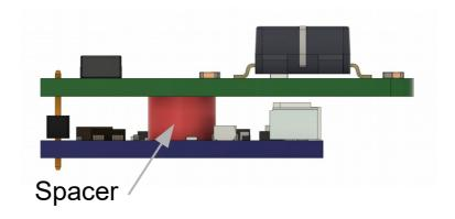
Fig.3 Spacers between boards
