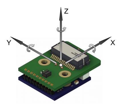
Fig.2 Measurement Axis and Directions
