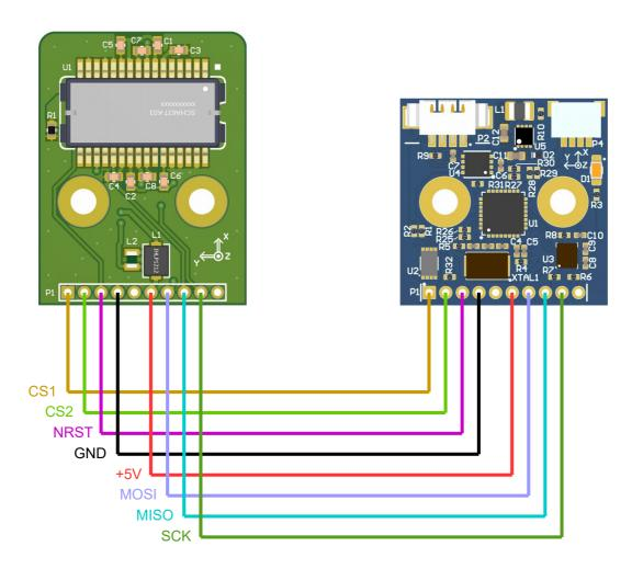
Fig.1 Connection between modules
